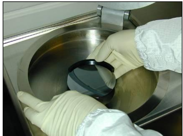
Fig. 4 – Centering a 4” wafer
