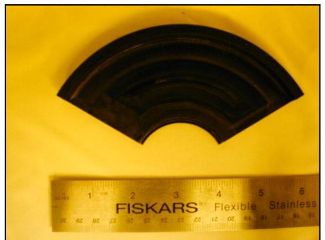
Fig. 8 – 6” wafer centering tool
