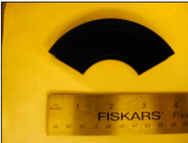
Fig. 7 – 4” wafer centering tool
